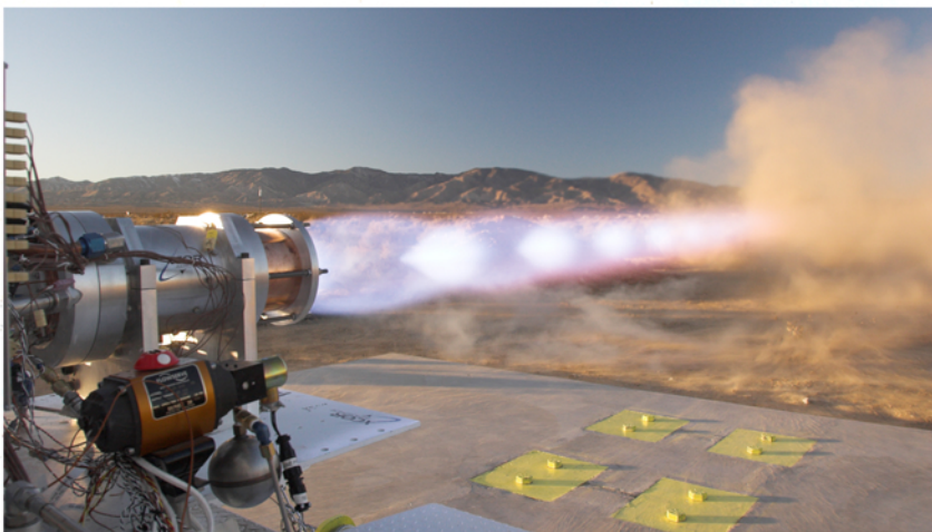
SHOCK-WAVE CONES emerge in the rocket plume of XCOR's methane-fueled engine, ground-tested last December. Such engines may power future spaceflight operations.
